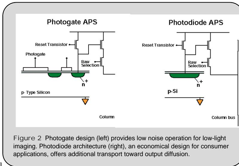
Figure 2 Photogate design (left) provides low noise operation for low-light imaging. Photodiode architecture (right), an economical design for consumer applications, offers additional transport toward output diffusion.
